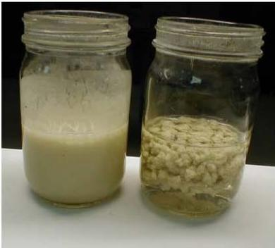
Tight Flocs Using Dual Flocculant Approach
