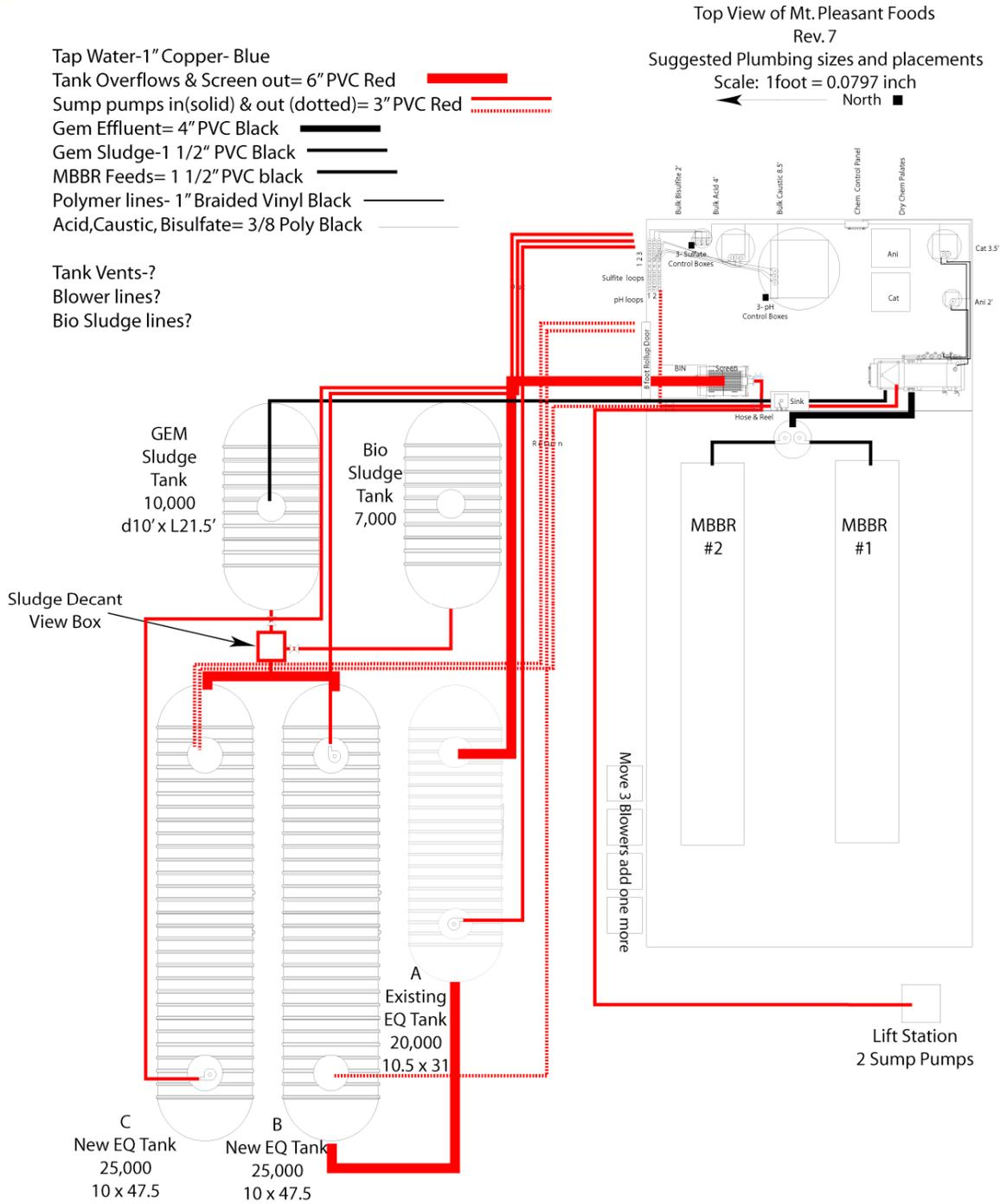
**Figure 3. Schematic Presentation of the System Installed to Treat WLF wastewater.**
