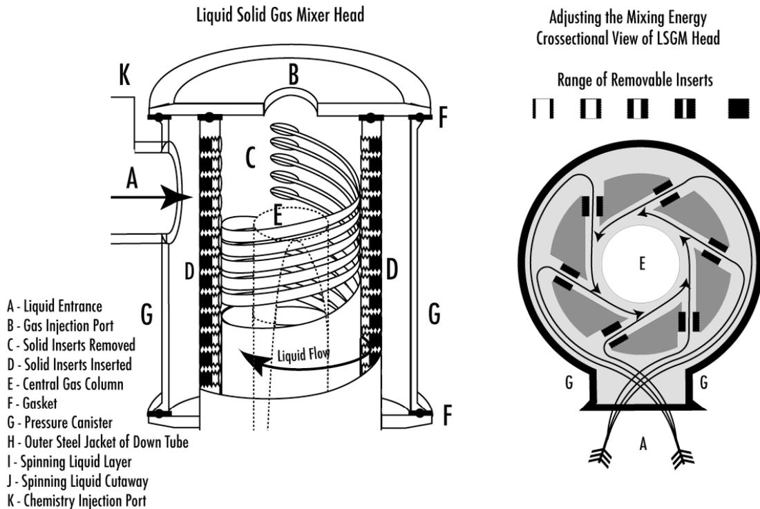
**Figure 5. Schematic Presentation of the LSGM Heads.**
