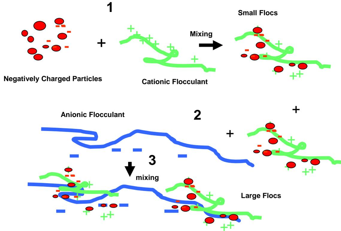
Figure 7. Dual polymeric flocculant approach.
