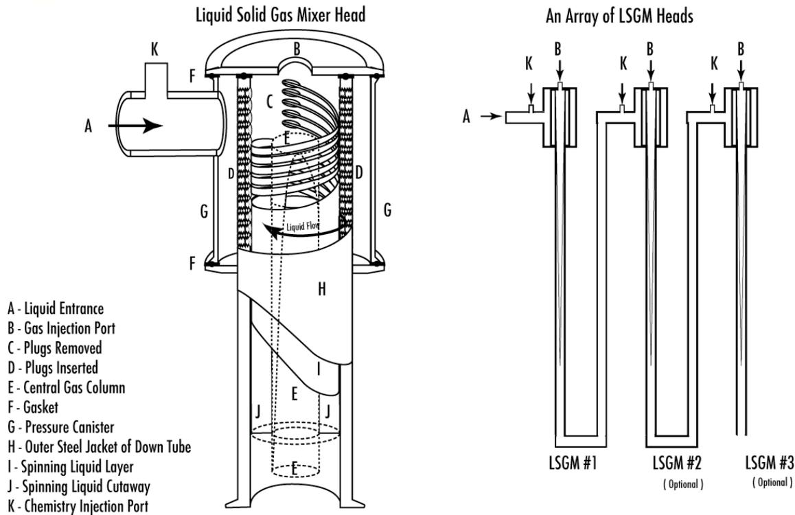
**Figure 4. Schematic Presentation of the LCP/LSGM.**
